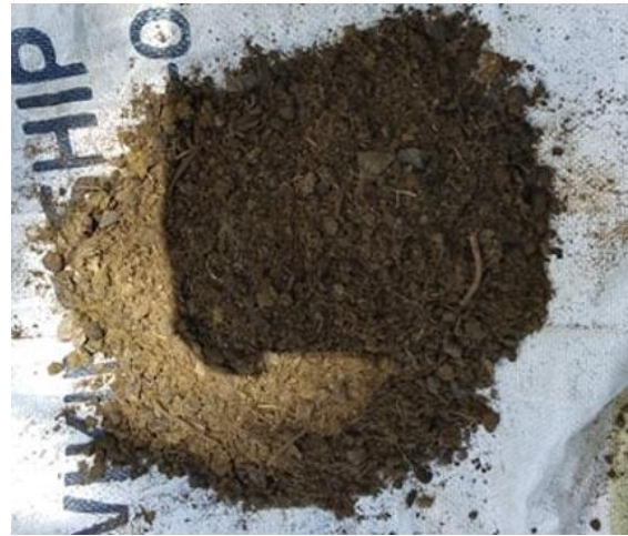
Fig. 2. Pulverized goat manure to be added to the concrete mixture.
