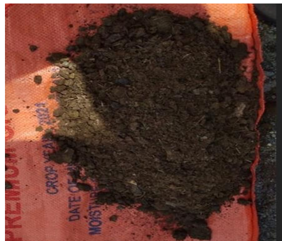
Fig. 3. Pulverized horse manure to be added to the concrete mixture.
