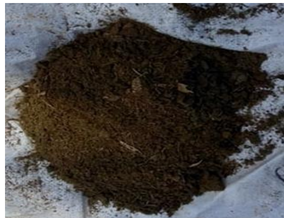
Fig. 4. Pulverized carabao manure to be added to the concrete mixture.
