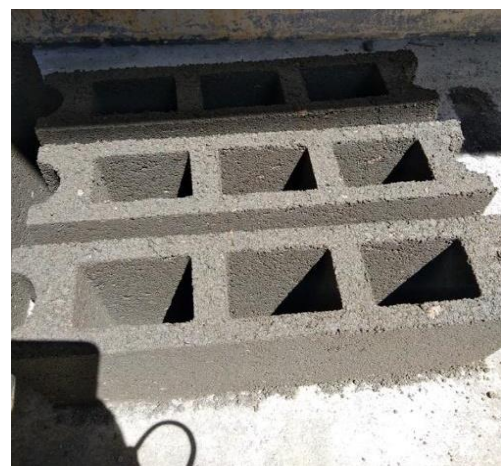
Fig. 7. CWCHB with 20g, 25g, 30g cow manure from top to bottom
