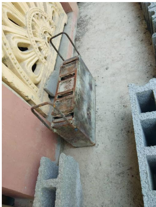
Fig. 5. Molder used for 40 cm length CHBs
