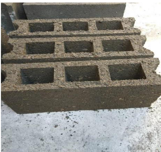
Fig. 10. CWCHB with 20g, 25g, 30g carabao manure from top to bottom
