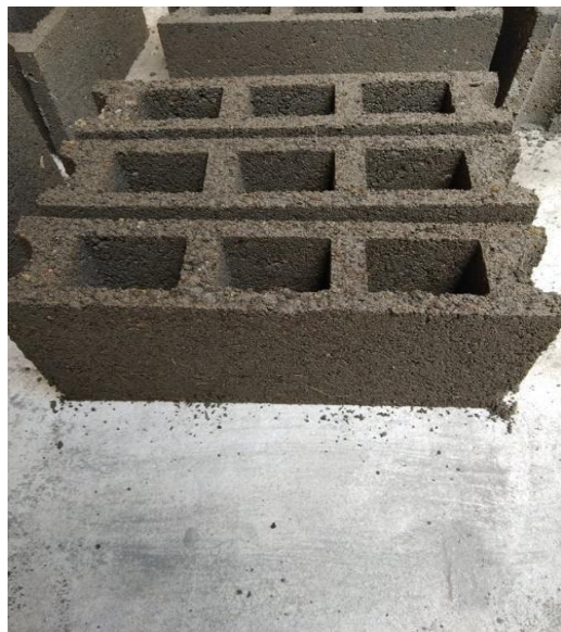
Fig. 9. CWCHB with 20g, 25g, 30g horse manure from top to bottom
