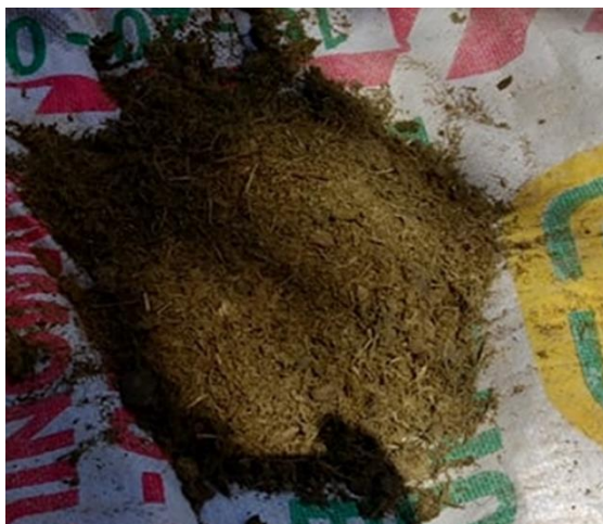
Fig. 1. Pulverized cow manure to be added to the concrete mixture.
